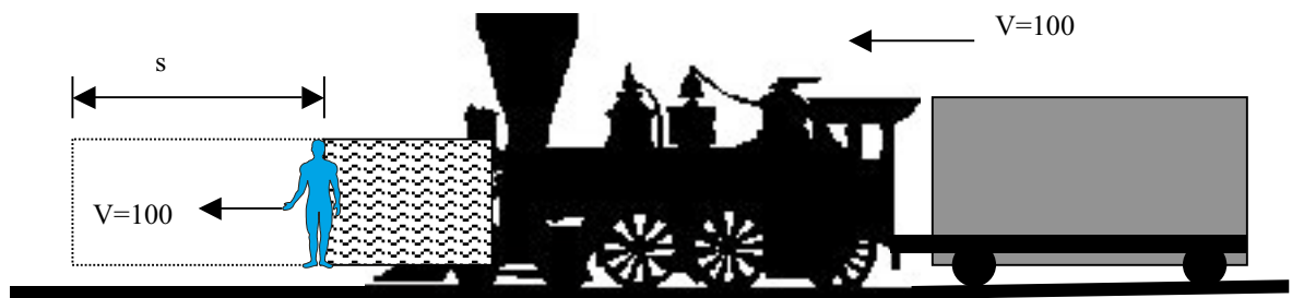
Figure 2b, impact between pedestrian and train with front airbag, after impact and deceleration distance 's'.
