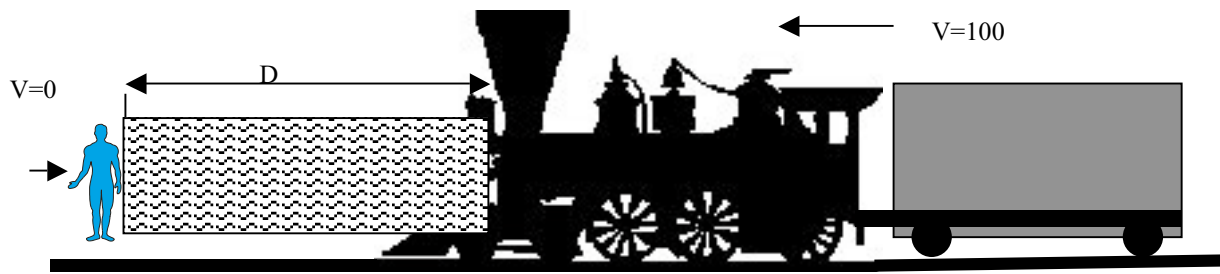
Figure 2a. At impact between pedestrian and train with front airbag.
