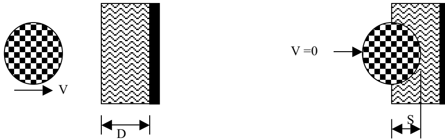
Figure 1 Diagram showing moving mass m (at speed V ) impacting a surface resulting in deformation S . D is the thickness of the material impacted.
