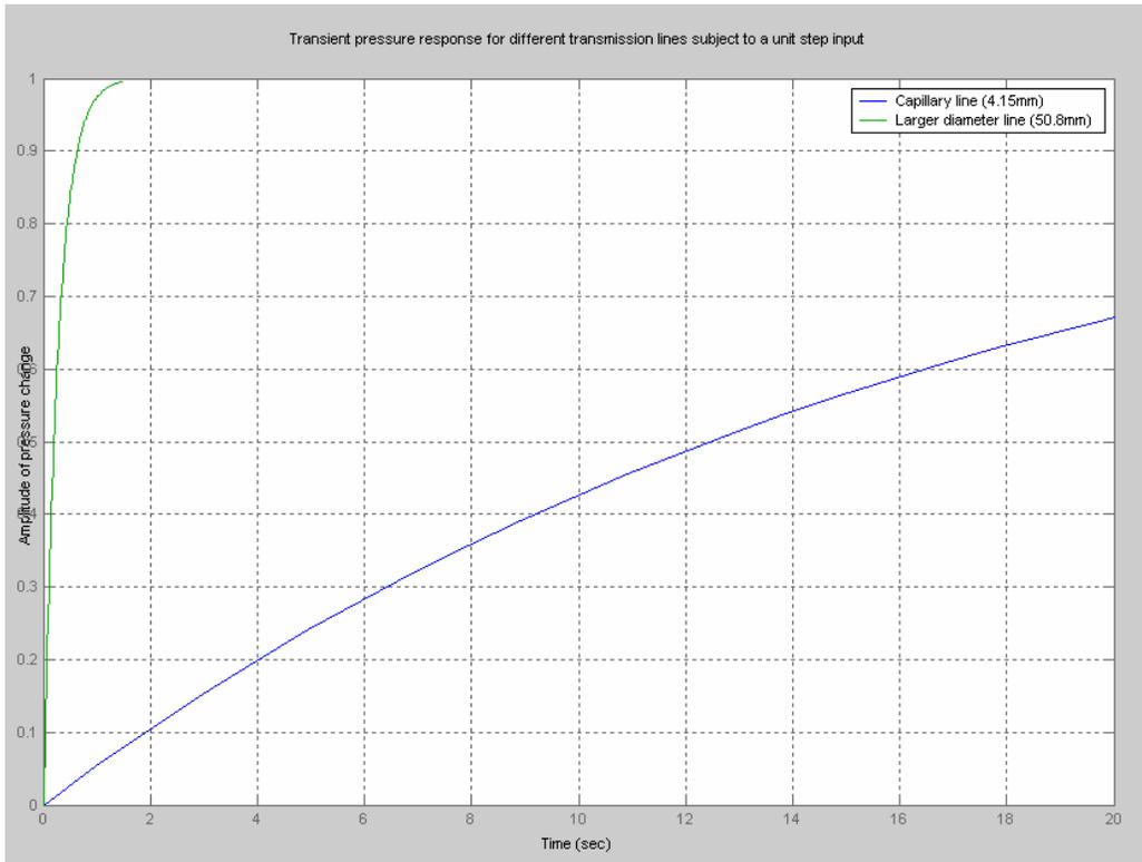
**Figure 2:** Transient pressure response for different transmission lines subject to a unit step input
