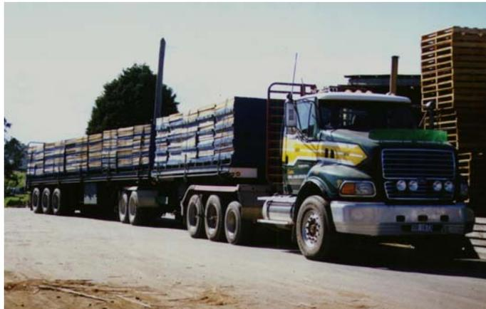
**Figure 4:** A B-double fitted with tri-axle group and the 50.8 mm diameter orifice transmission line
