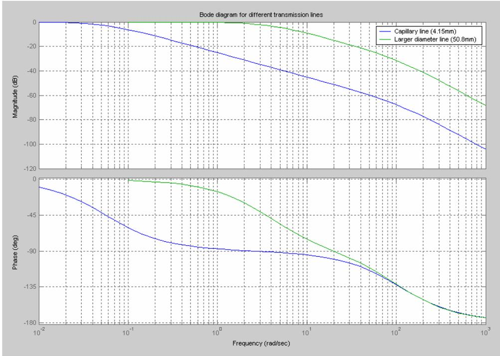
**Figure 3:** Frequency response for different transmission lines
