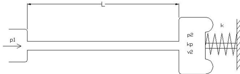
**Figure 1:** Simplified transmission line physical model [6]
