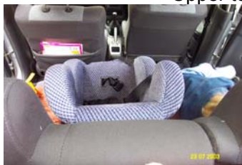
No Upper tether visible
