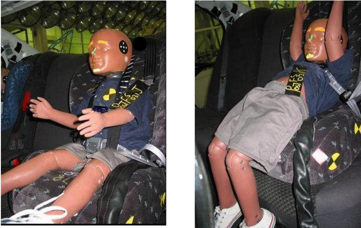
**Figure 5. Frontal test for Booster A with seatbelt and harness with crotch strap (left) and with the crotch strap disengaged (right)**
