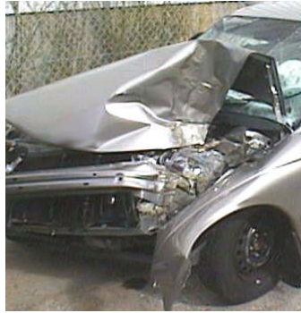
(b) Case 1: Target vehicle showing pole impact.
