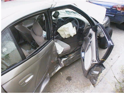
(a) Case 1: Target vehicle showing the lateral impact.
