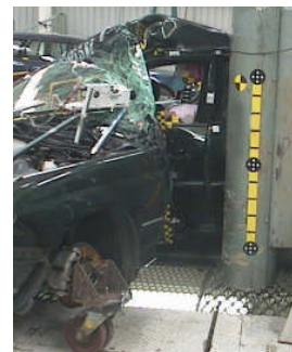
(f) Case 3: Target vehicle showing impacted pole.
