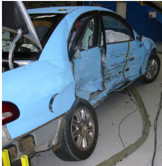
(a) Case 1: Target vehicle showing the lateral impact
