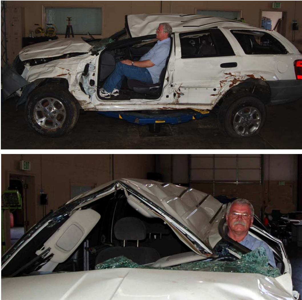
Figure 1: Tenting roof crush and pillar deformation leaves little room for survival
