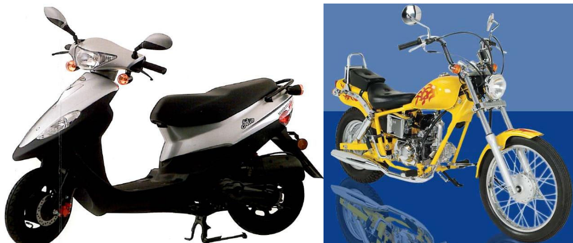
Figure 1: Mopeds – scooter style (step through) on left is most common but can be motorcycle-style (step over) as shown on right.
