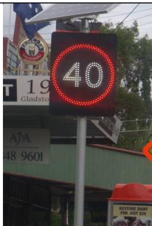
Variable speed limit sign (installed in conjunction with static school zone sign)
