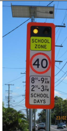
Enhanced School zone speed limit sign (flashing light school zone sign)
