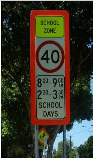
Static school zone speed limit sign (also installed in advance of signs shown below)
