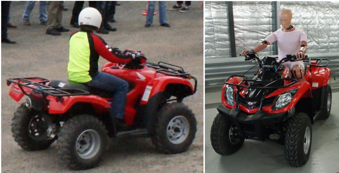
Figure 1: Quad bike similar to motorcycle regarding vehicle operation, that is operator sits in straddle position, using handlebars to steer vehicle, throttle is usually on the right arm of the handlebar and brakes are on both sides of the handlebars.
