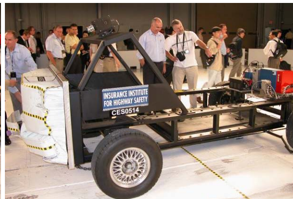
Jack Haley (NRMA) pointing out features of the IIHS's elevated movable crash barrier to Michael Case (RACV) with Lauchlan McIntosh (AAA) in the background looking on.
