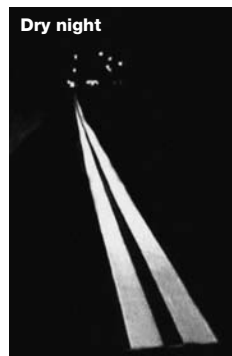
Dry night Conventional painted pavement marking (left), and VisiBead® pavement marking (right).
