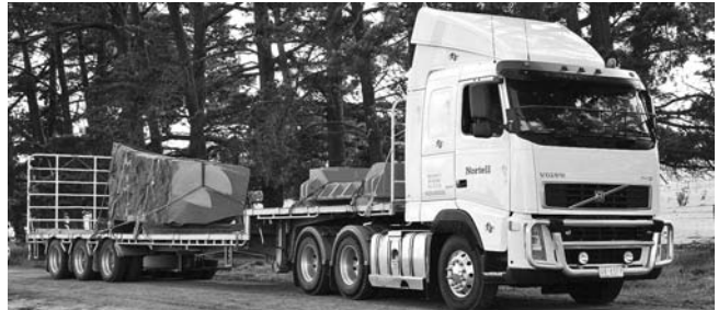
Figure 4: Trawalla level crossing - reconstruction showing a similar semi-trailer and the load involved in the level crossing crash. Note the extreme collision interface incompatibility between the front of the high speed train and the trailer and large 'rock' impacted.
