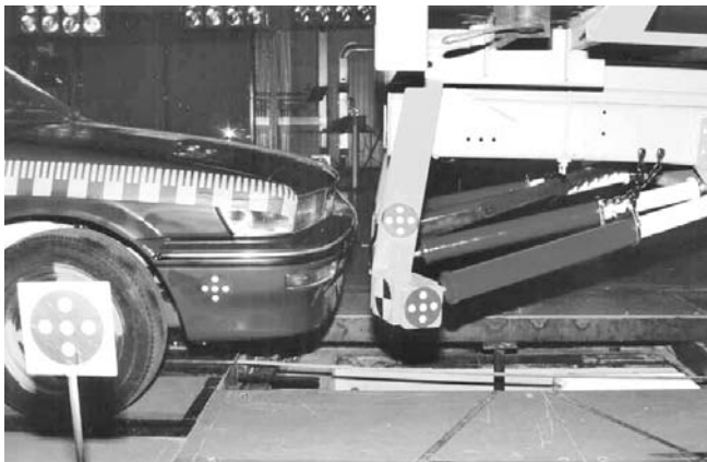
Figure 7 Detail showing interface height of front of Corolla and the underrun barrier.
