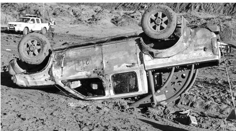
Figure 9: (Above Middle & Bottom) Third rollover of a vehicle equipped with Swan ROPS resulting in maintenance of occupant survival space and only minor injuries.
