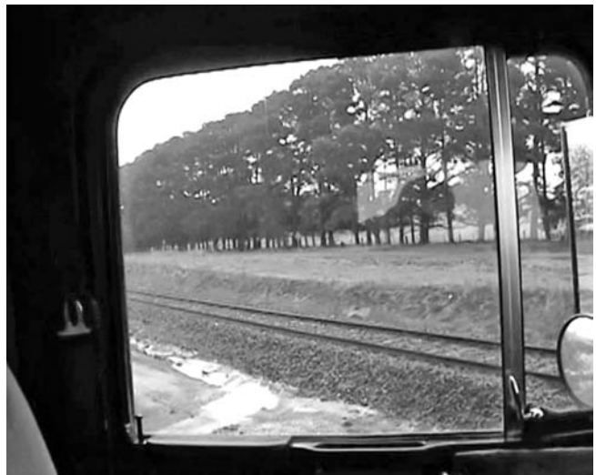
Figure 5: Trawalla level crossing - reconstruction showing the view from the driver's seat and the severely restricted length of track able to be seen. This is an example of very poor visual interface design at the crossing, arising from the level crossing design and the prime-mover cabin design.
