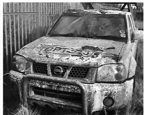
Figure 9: (Above Middle & Bottom) Third rollover of a vehicle equipped with Swan ROPS resulting in maintenance of occupant survival space and only minor injuries.
