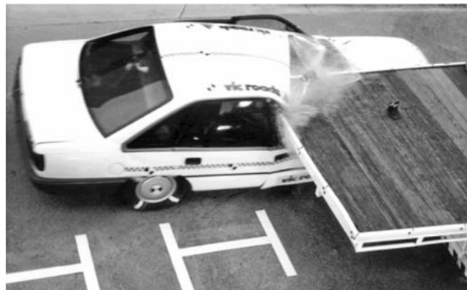
Figure 6: Rear underrun crash test of commodore sedan at 50km/h into rear of tray truck without an underrun barrier)
