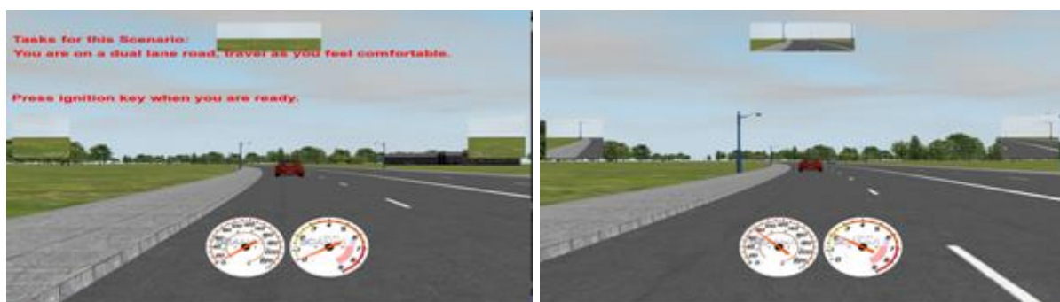
Figure 2. The screen shot on the left shows the start of the overtaking scenario with instructions. The overtaking scenario in progress is shown on the right. The car ahead is the IV.
