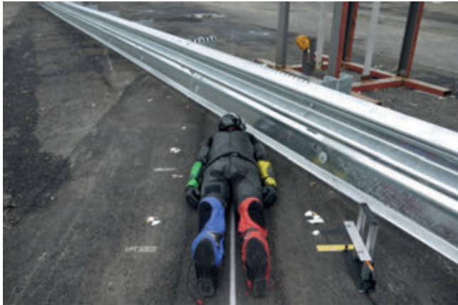
Figure 5. Set up used in the motorcyclist crash tests
