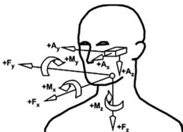
F_x - anterior-posterior shear force, F_y - lateral shear force. F_z - tension-compression force, M_x - lateral bending moment on the neck, M_y - flexion/extension moment on the neck, M_z - torsion moment ( M_z ).
