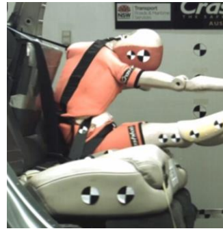
Figure 8: Lap belt position during the impact phase, TNO P10, Stage 1 integrated booster, CREP pulse
