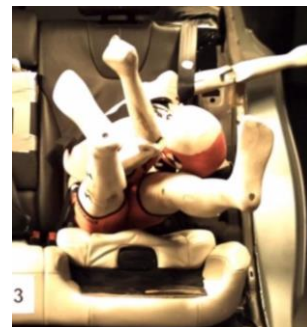
Figure 4: Sash belt slips from the shoulder at point of maximum forward excursion, TNO P10, Stage 1 integrated booster, CREP pulse
