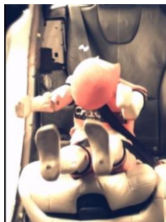
Figure 3: Sash belt remains in contact with the shoulder at point of maximum forward excursion, TNO P6, Stage 2 integrated booster, CREP pulse
