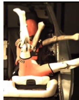
Figure 6: Sash belt remains in contact with the shoulder during rebound, TNO P10, Stage 1 integrated booster, CREP pulse
