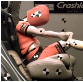
Figure 7: Lap belt position during impact phase, TNO P6, Stage 2 integrated booster, CREP pulse
