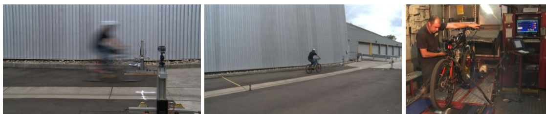
Figure 5. Tests showing (L-R) speed sensor setup; brake testing; and dynamometer setup for 48cc unrestricted petrol-powered bicycle
