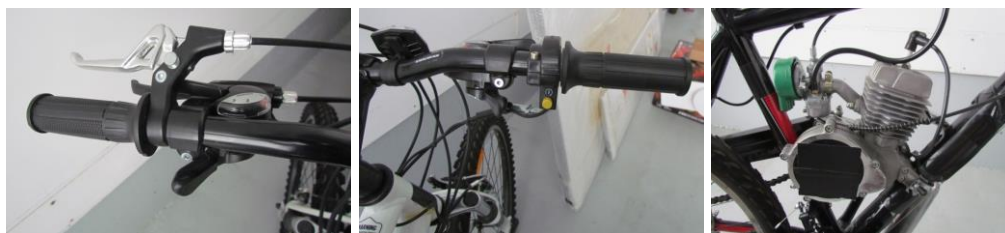
Figure 3. Setup for 48cc petrol-powered bicycle showing (L-R) silver clutch lever above the standard brake lever on the left handlebar; the right grip modified as a throttle; and the motor – note the exposed engine and components, including fuel lines and drive chain
