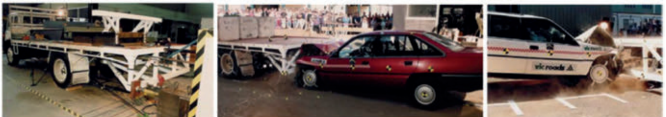
Figure 3. RUPD rigid barrier design (Rechnitzer, Powell & Sayer, 2001)
