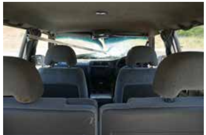
Figure 2. Test 1 – sign layout & vehicle damage after crash
