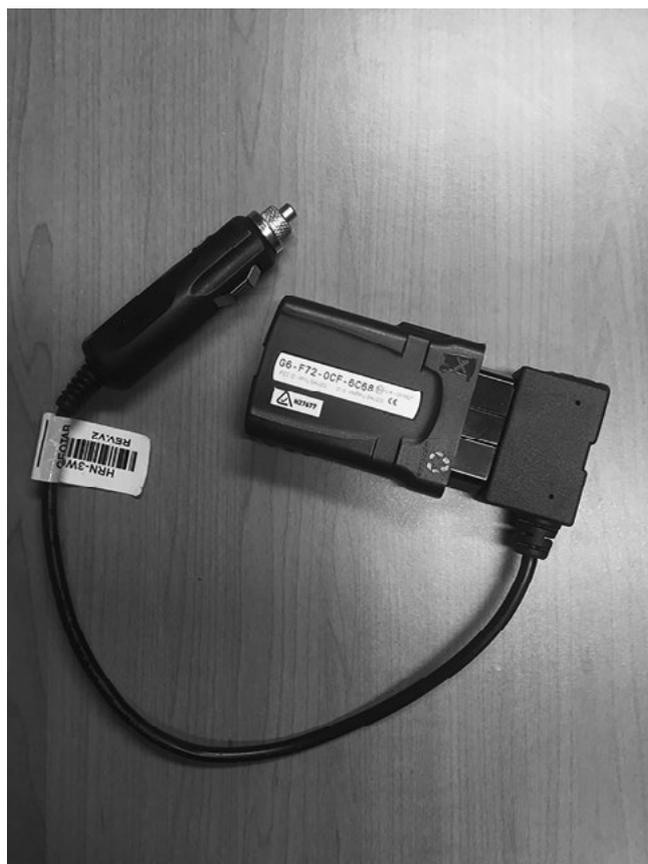
Figure 1. In-vehicle driver monitoring device
