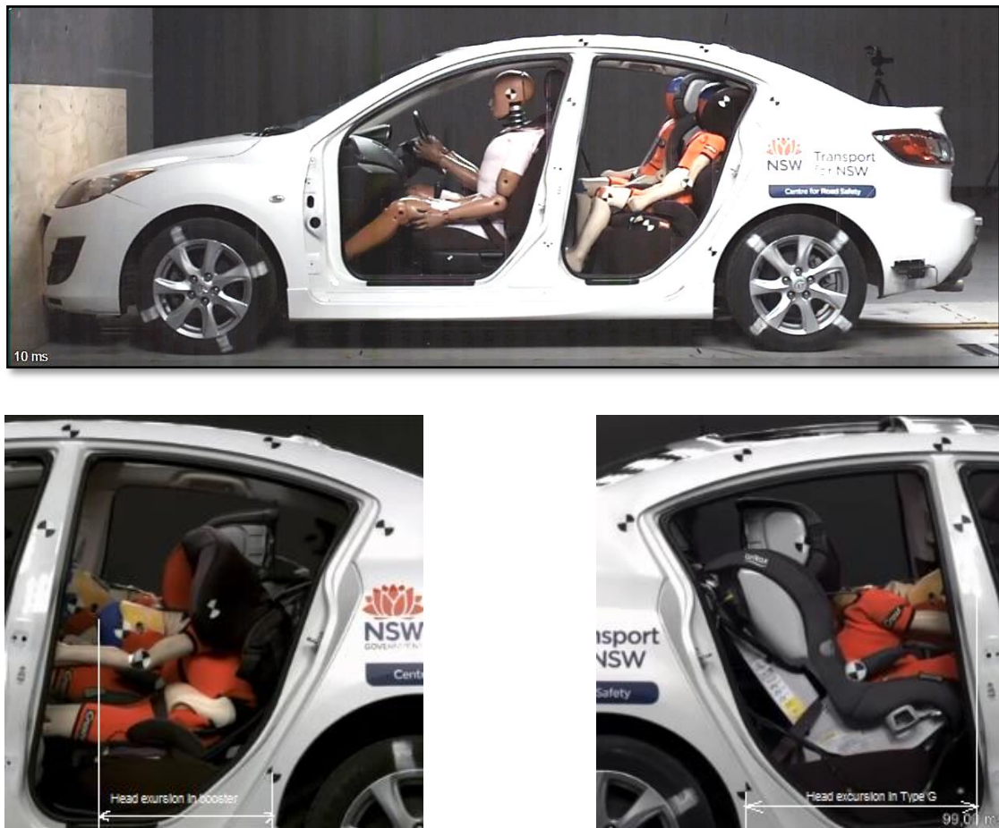
Figure 1. Test Setup (above) and head excursion results for dummy in Type-G (bottom right hand side) and dummy in booster seat (bottom left hand side)
