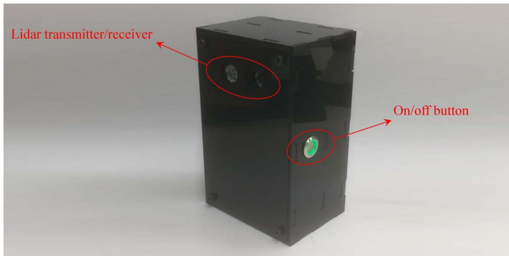
Figure 1. LIDAR lane position and lateral offset measurement device
