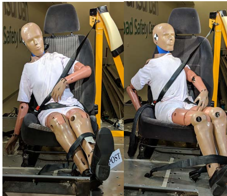
Figure 1. Post-crash belt position for the baseline test (left) and lumbar support roller (right) showing the belt intruded into the abdomen when using the lumbar support roller
