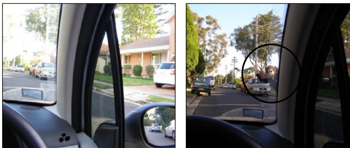
Figure 4: Example of poor visibility from vehicles showing pedestrian standing close to the vehicle is completely obscured by the A pillar
