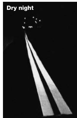
Dry night Conventional painted pavement marking (left), and Visibead® pavement marking (right).
