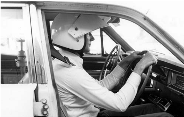
Figure 3. The 'snapping turtle' occluding helmet was used to test delineation treatments by periodically interrupting drivers' vision and seeing how well they could stay on path. Note the dual controls in the car – just in case!
