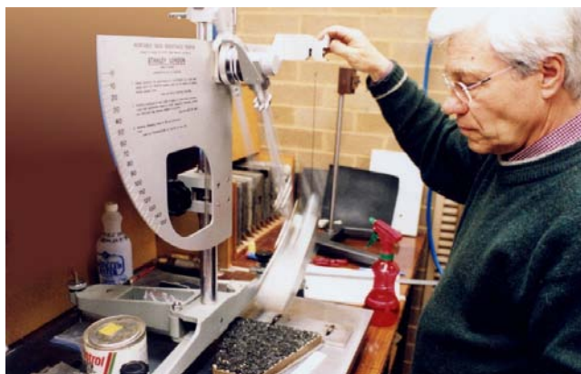
Figure 4. A British Pendulum Tester being calibrated in the laboratory. This was (and still is) used to measure skid resistance.
