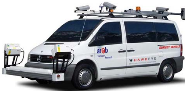
Figure 5. A network survey vehicle equipped with Hawkeye video cameras are mounted on the roof. The apparatus at the front of the van is a battery of laser sensors for measuring road surface characteristics.
