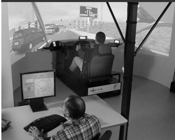
Drivers are ideally prepared for critical traffic situations and learn how to handle safely situations, which cannot, or can only conditionally, be practised on public roads. The basic RDE modules make it possible to reproduce practically all possible road and driving conditions in high-fidelity virtual mode.
