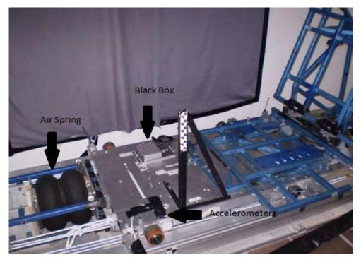
Figure 3: Low-speed impact crash test sled
