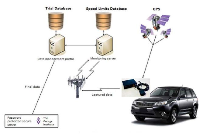
**Figure 2: Data transmission via the telecommunications network** (adapted from [Greaves, Fifer et al. 2010])
