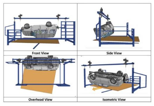
Figure 2. Modelled JRS test setup with Ford Explorer
