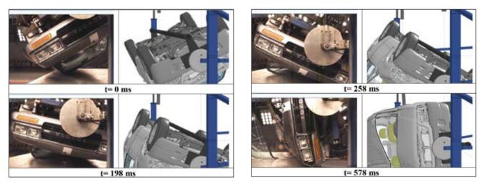
Figure 3. Sequence of test with SUV vehicle - comparison between test (left) and simulation (right)
