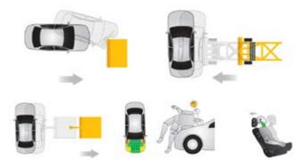
Figure 1. The range of ANCAP current testing
