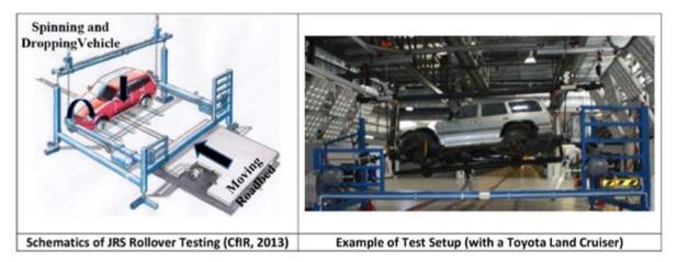
Figure 1. Schematic of JRS rollover testing rig and example of an actual test setup
