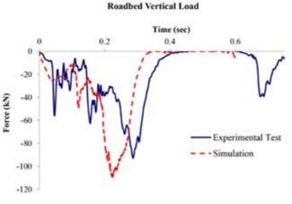
Figure 6. Roadbed vertical load - comparison between experimental test and simulation
