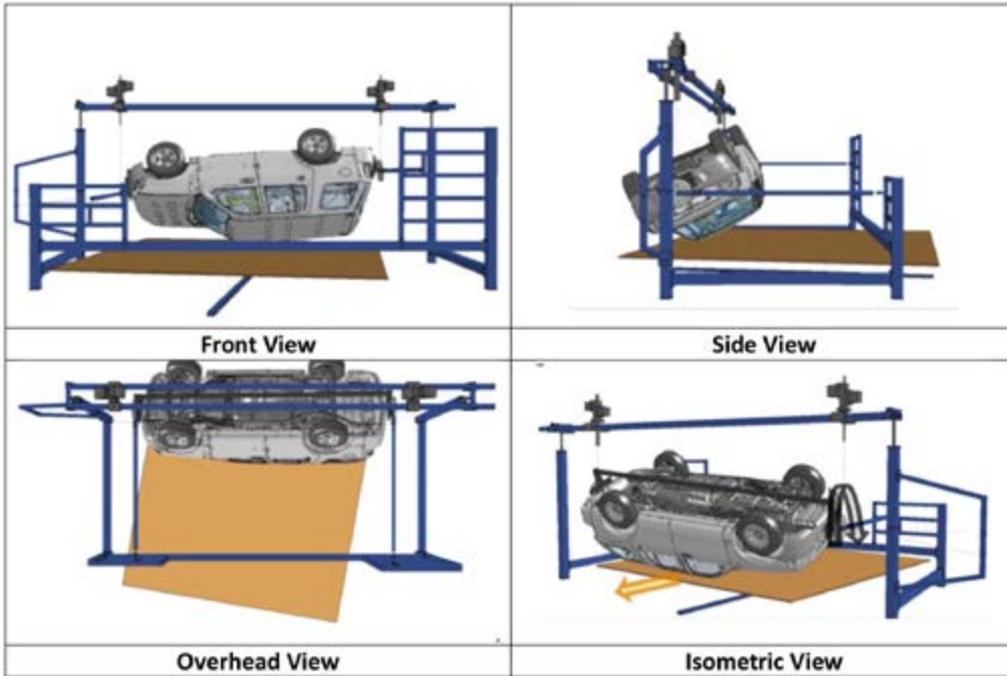
Figure 2. Modelled JRS test setup with Ford Explorer
