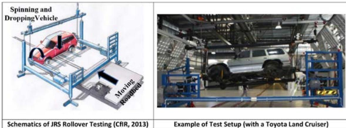
**Figure 1. Schematic of JRS rollover testing rig and example of an actual test setup**
