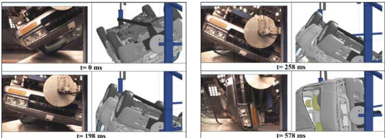
Figure 3. Sequence of test with SUV vehicle - comparison between test (left) and simulation (right)
