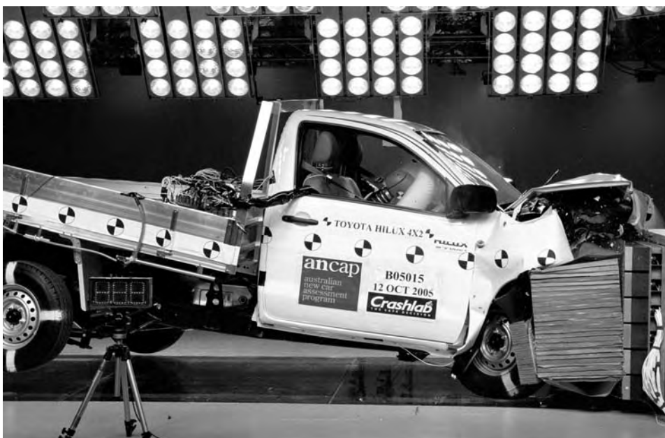
A recent ANCAP offset frontal crash test of a Toyota Hilux 4x2 ute conducted at 64km/hr. The Hilux scored 4 stars in this test.
