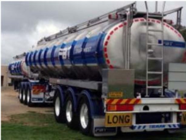
Photographs showing day and night images of an FBT Transwest tanker with high visibility reflective markings.
