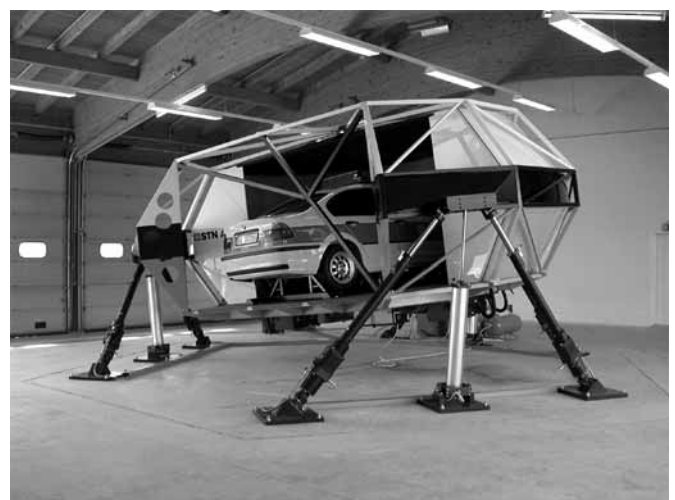
Fig. 1: High-End-Simulator with 6-legs movement system. En route to the destination all inertia forces are simulated.
