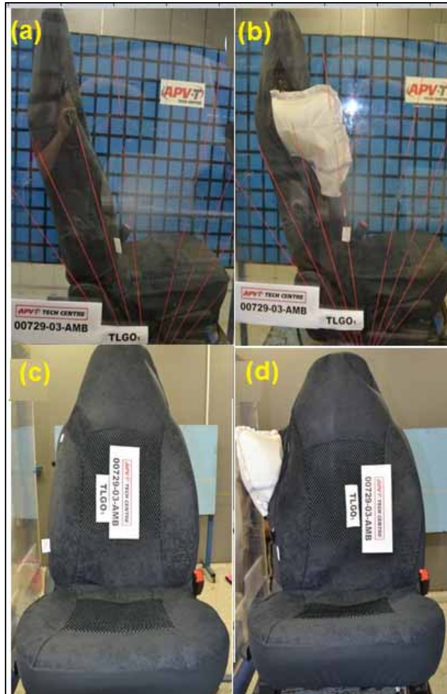
Figure 4 Airbag deployment testing (a) side view before deployment (b) side view after deployment (c) front view before deployment (d) front view after deployment
