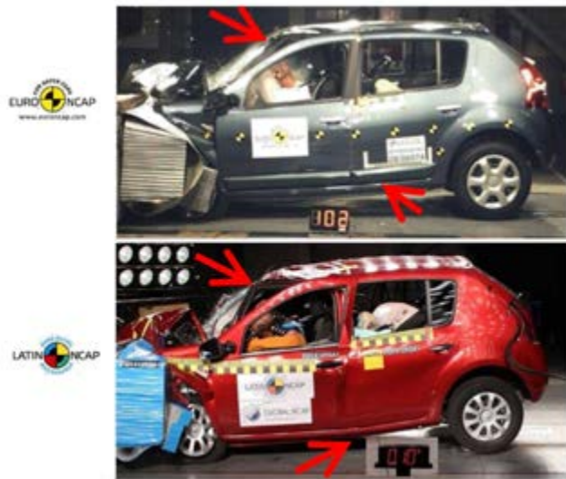
Sandero: Comparing the same model from different plants, the difference in bodyshell stability can be clearly noticed.
