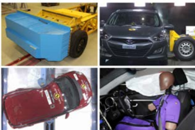
Figure 1. In 2015, the Euro NCAP side impact crash tests will be updated with new elements such as the Advanced European Mobile Deformable Barrier (AE-MDB) and the WorldSID mid-sized male dummy.
