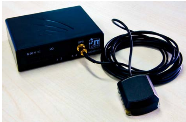
Figure 1: In-vehicle monitoring device (11cm x 8.5cm x 3cm)
