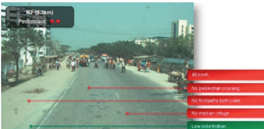
Figure 5. A section of Highway N2 rated 2 stars for pedestrians
