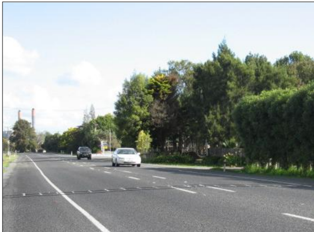
Figure 3: Vehicle position survey with speed recording tube counters
