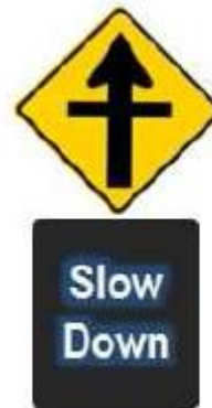
Figure 8: Proposed slow down intersection active warning trial sign
