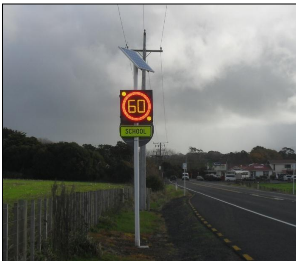
Figure 5: 60km/h variable speed limit school trial sign on State Highway 23 at Te Uku School (within permanent 80km/h speed limit).
