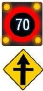
Figure 7: Proposed 70km/h variable speed limit intersection active warning trial sign
