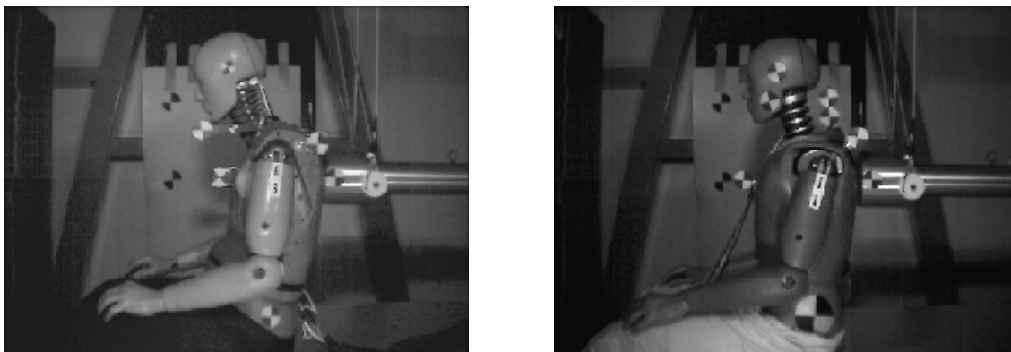
Figure 4. Initial dummy position and film marker position for the BioRID (left) and Hybrid III (right).
