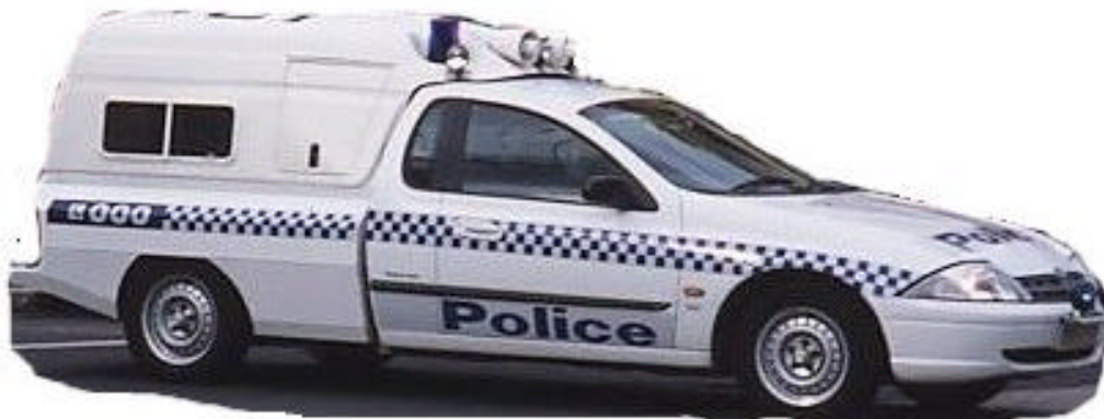
Figure 5. The Interim Ford Falcon AU Divisional van with much improved rollover stability characteristics, based on a Ford Falcon utility fitted with a modified prisoner pod from the previous Commodore van.
