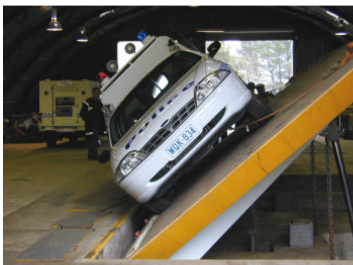
Figure 3. View showing a Police vehicle undergoing Tilt-Table test at the Army’s Monegetta test facility
