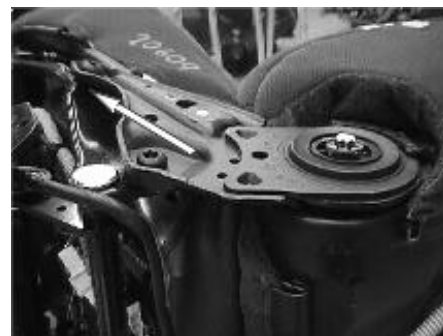
Figure 5. Deformation on the cushion in the Saab seat (609), which allows the reclining of the seat back.
