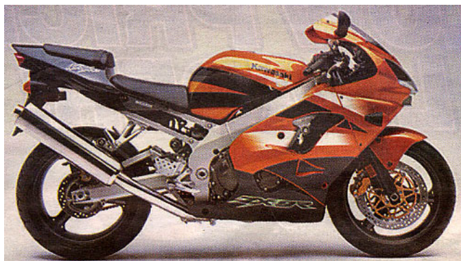
KAWASAKI ZX – 9R - 900 cc: Cost: $17990 + ORC; Power – 105 kW; weight – 186 kg; Power to weight ratio – 380 with 90 kg of rider, fuel etc; Acceleration – 0-100 km/h – 2.9 sec; top speed – 276 km/h
