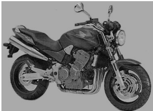
HONDA HORNET CB900F - 900 cc: Cost: $13990 + ORC; Power – 80 kW; weight – 194 kg; Power to weight ratio – 282 with 90 kg of rider, fuel etc; Acceleration – 0-100 km/h – 2.9 sec; top speed – 228 km/h
