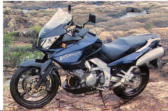
SUZUKI V-STROM DL - 1000 cc: Cost: $15490 + ORC; Power – 72 kW; weight – 207 kg; Power to weight ratio – 242 with 90 kg of rider, fuel etc; Acceleration – 0-100 km/h – 3.4 sec; top speed – 200 km/h
