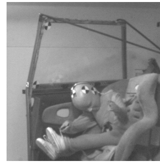
Incorrect harness use with forward facing CRS
