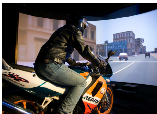
Figure 1: Riding simulator set-up for motorcycle rider hazard perception experiment.
