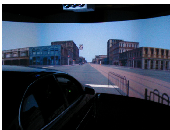
Figure 2: Driving simulator set-up for car driver hazard perception experiment.
