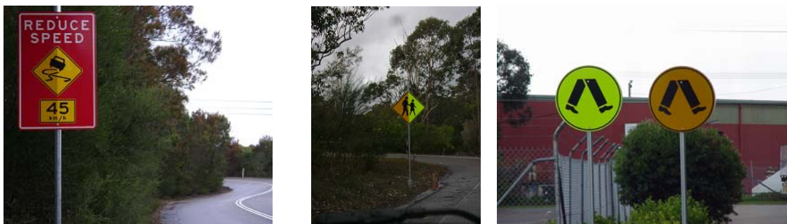
Figure 1 – Warning sign and pedestrian signs prepared with standard and fluorescent sheeting.
