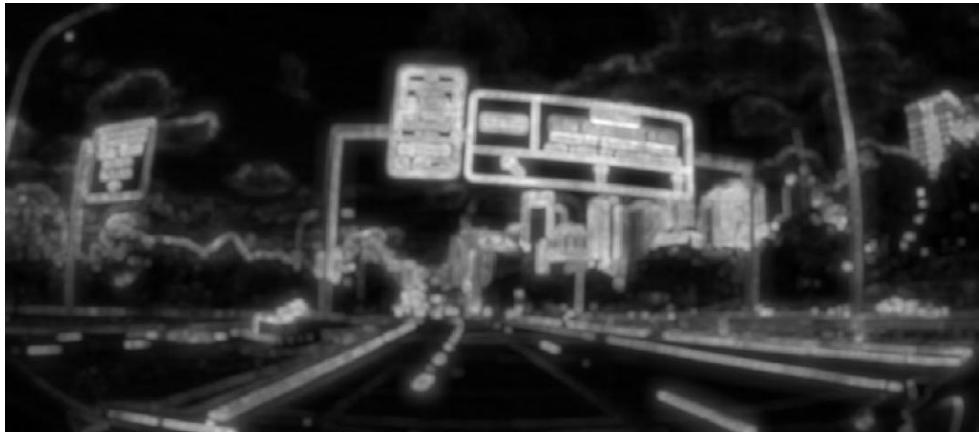
Figure 2. Example of feature congestion clutter map using Figure 1 ('hotspots' indicate areas of relatively high clutter)
