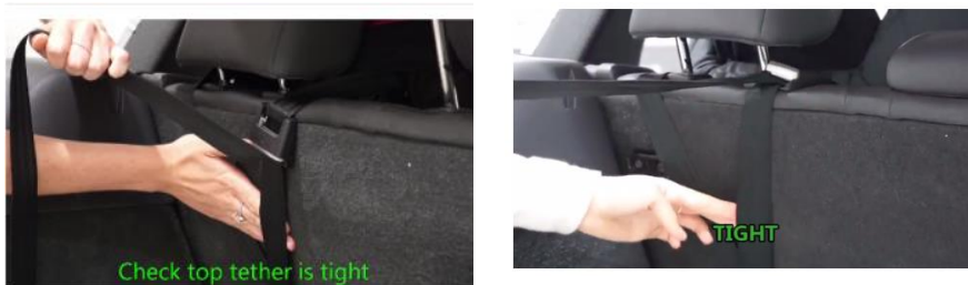
Figure 3. Modification to address tether strap slack, round 1 (left) versus round 2 (right)
