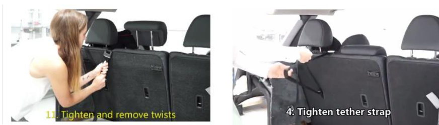
Figure 2. Modification to address tether strap slack, round 1 (left) versus round 2 (right)
