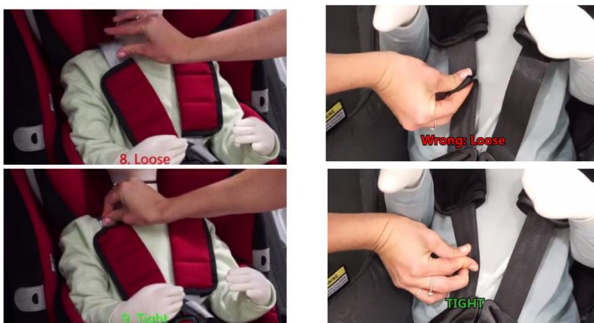
Figure 4. Modification to address harness strap slack, round 1 (top left, bottom left) versus round 2 (top right, bottom right)
