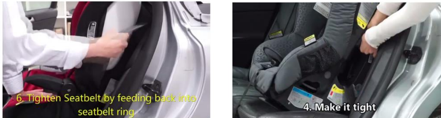
Figure 1. Modification to address seatbelt slack, round 1 (left) versus round 2 (right)
